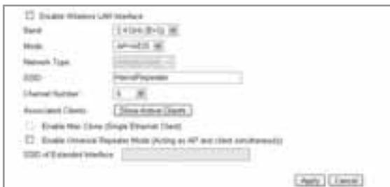
The selection under **Band** allows you to specify whether the device runs in the 2.4 GHz band in accordance with the 802.11b (11Mbps), 802.11g (54Mbps) standard or works in combination with 802.11b and 802.11g.
